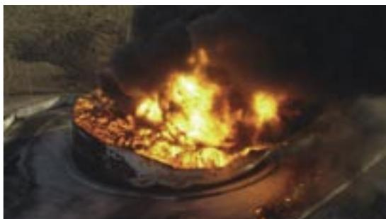
Fig 7.1 - Fixed Roof Tank Full Surface Fire (Full Roof Removal).
